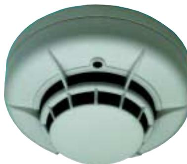
**The ECO1003 photoelectric smoke detector's** chamber has been specifically designed to be highly tolerant to the long term build-up of dust and other airborne contaminants. This high level of immunity significantly reduces the potential for unwanted alarms caused by settled dust increasing the detector's sensitivity. Additional immunity to unwanted alarms arising from short-lived transients is also provided through the use of special signal processing.
