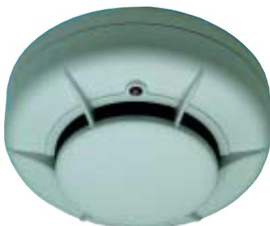
**The ECO1003 photoelectric smoke detector's** chamber has been specifically designed to be highly tolerant to the long term build-up of dust and other airborne contaminants. This high level of immunity significantly reduces the potential for unwanted alarms caused by settled dust increasing the detector's sensitivity. Additional immunity to unwanted alarms arising from short-lived transients is also provided through the use of special signal processing.
