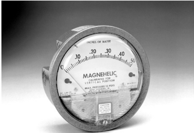
Figure 14: Magnehelic gauge for reading static pressures in air systems
