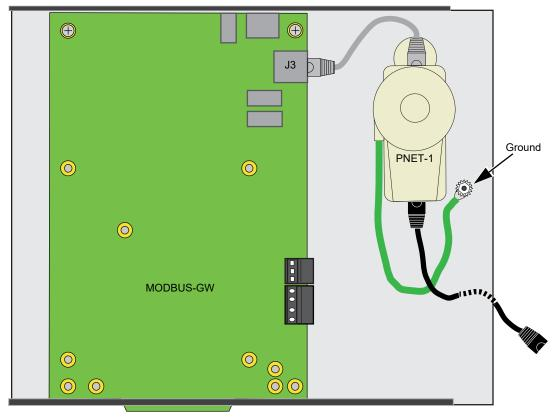
Figure 9. Connecting to the PNET-1
