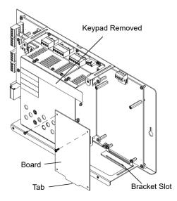
Install bracket on 1/2" standoffs. Place the board's tab in the bracket slot and screw the board to the top of the standoffs. May be stacked in front of or behind another board using standoffs of adequate length to clear the rear board.
