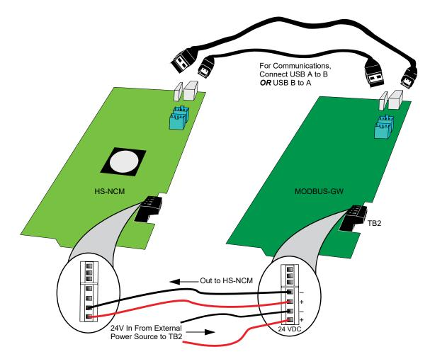
Figure 7. Routing Power and Communication to an HS-NCM
