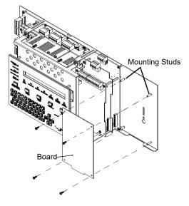
Mount in 4th column of the NFS2-640 Series chassis. Mount chassis to backbox before installing the board in rear position. May be mounted in front of another board using standoffs of adequate length to clear the rear board.
