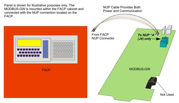
Figure 8. Connecting to an FACP
