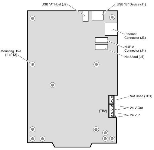
Figure 5. MODBUS-GW Connections
