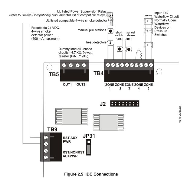
Input Circuits Installation
