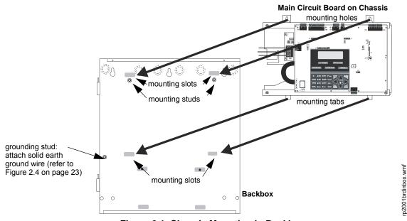
Figure 2.1 Chassis Mounting in Backbox
