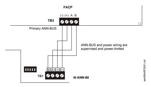
Figure 2.18 FACP wiring to ANN-BUS Device
