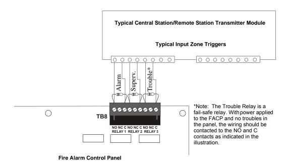
Figure C.5 FACP Dry Contacts Connection to Central Station/Remote Station Transmitter
