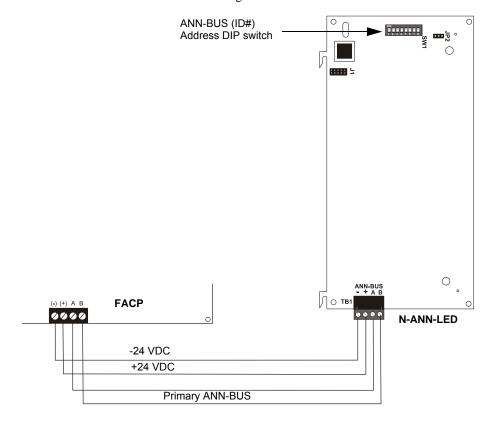
Figure 2.25 N-ANN-LED Board Layout and Connection to FACP
