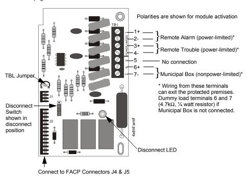
Figure 2.16 4XTM Transmitter Module
