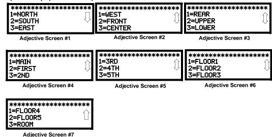
Pressing 2 while viewing the Adjective/Noun Screen will cause the following screen(s) to be displayed. Note that the keyboard *down* arrow key must be pressed to see all the Noun screens. Press the number corresponding to the noun that is to be used as a descriptor for the location of the detector currently being programmed. When a noun has been selected, it will appear at the top of the display as indicated by the asterisks.
