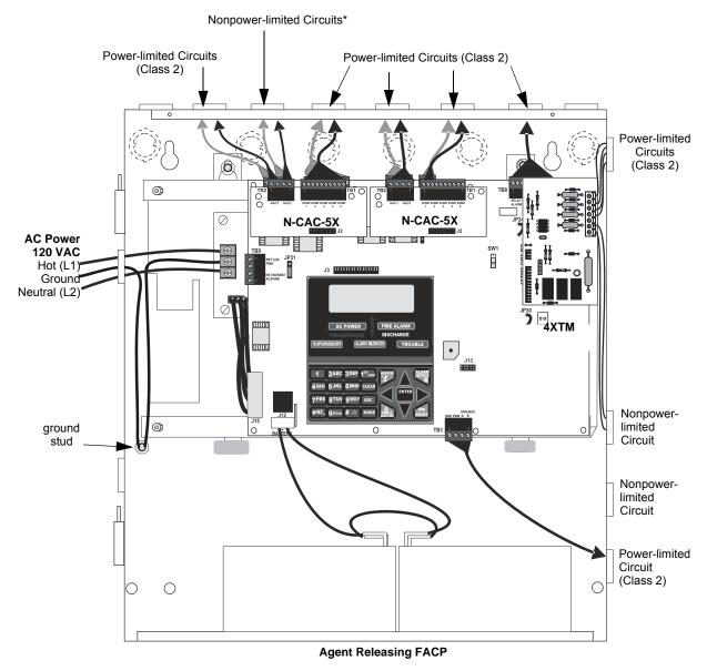
Figure 2.12 Typical UL Power-limited Wiring Requirements
