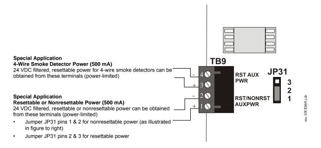
Figure 2.10 Special Application Auxiliary Power
