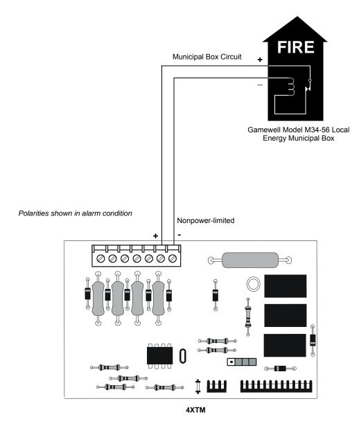
Figure C.2 Municipal Box Connected to 4XTM Transmitter Module
