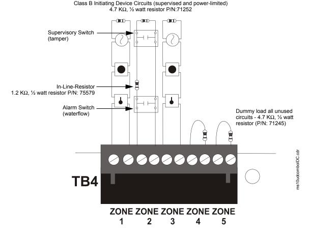
Figure 2.6 Style B Combination Circuit on Zone 2
