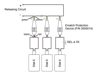
Figure 2.9 Wiring Stat-X Devices
