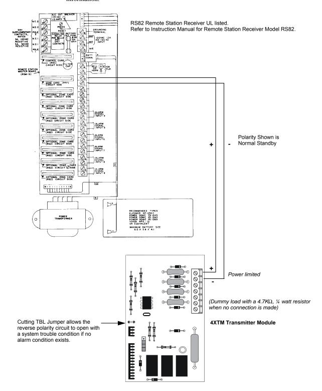
Figure C.3 Remote Station Connection Using 4XTM Module
