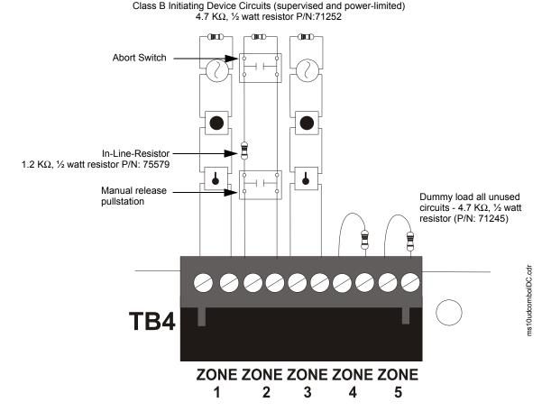
Figure 2.7 Style B Combination Circuit on Zone 2
