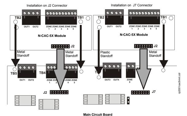
Figure 2.13 N-CAC-5X Module Installation
