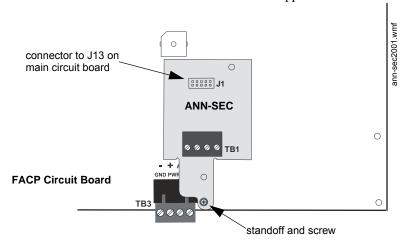
Figure 2.17 Installing the ANN-SEC Option Card
