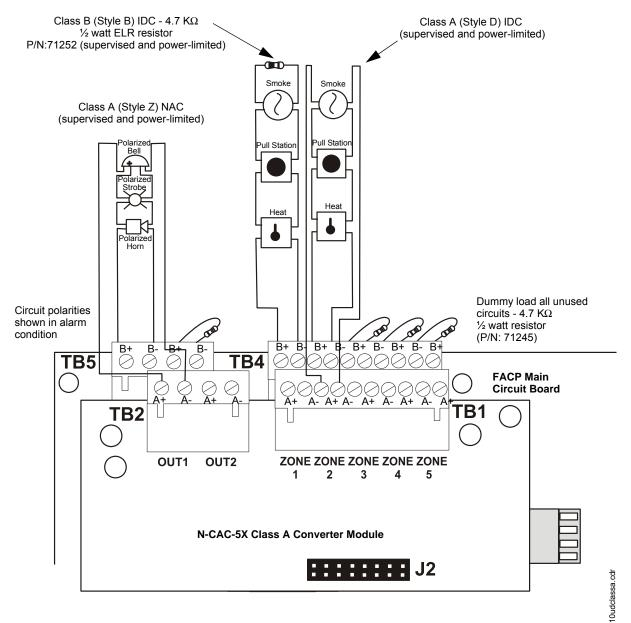
Figure 2.14 Wiring NACs and IDCs for Class A Operation
