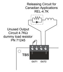
Note: Short Circuit Supervision must be enabled when using the REL-4.7K for Canadian Applications. Refer to the section titled "Release Circuit 1 or Release Circuit 2" on page 59 for information on enabling short circuit supervision.
