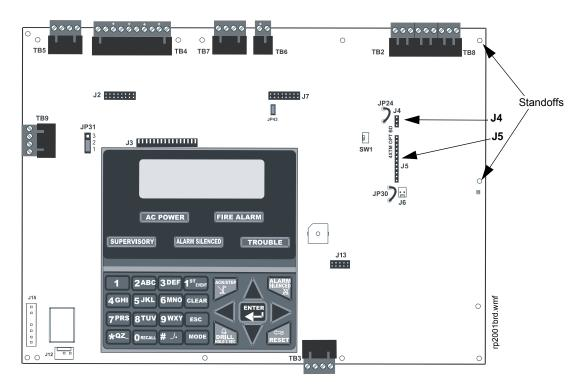
Figure 2.15 4XTM Option Module Connection
