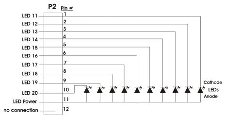
Figure 2.24 N-ANN-I/O LED Wiring
