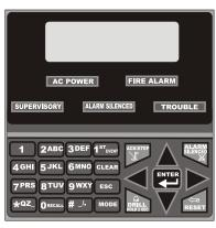
Figure 1.3 Membrane/Display Panel
