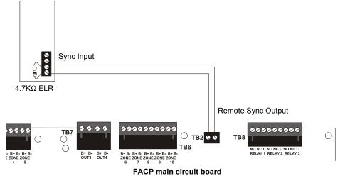
Figure 2.10 Remote Sync Output
