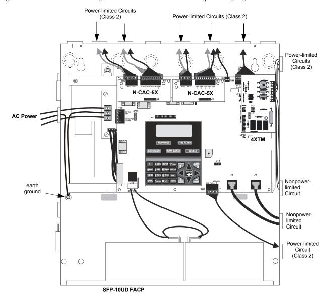
Figure 2.11 Typical UL Power-limited Wiring Requirements
