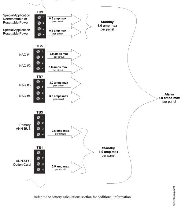
Figure 1.2 Current Availability with FACP and FLPS-7 Power Supply
