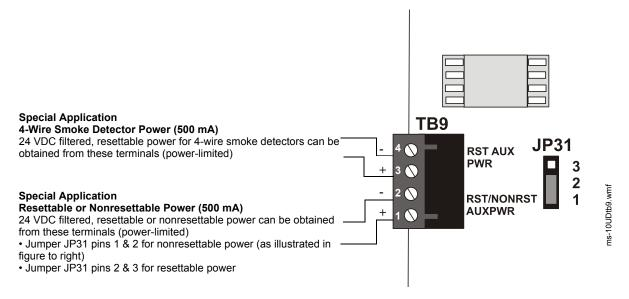
Figure 2.8 Special Application Auxiliary Power
