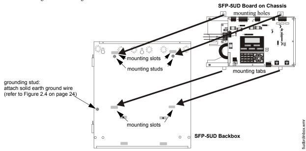
Figure 2.1 Chassis Mounting in Backbox
