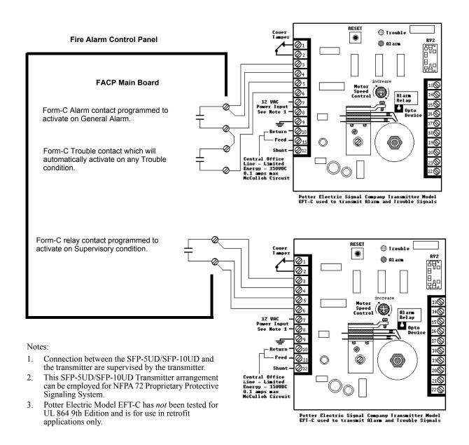
Figure B.4 Proprietary Protective Signaling System
