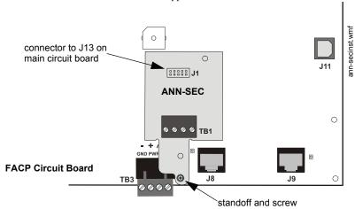
Figure 2.18 Installing the ANN-SEC Option Card
