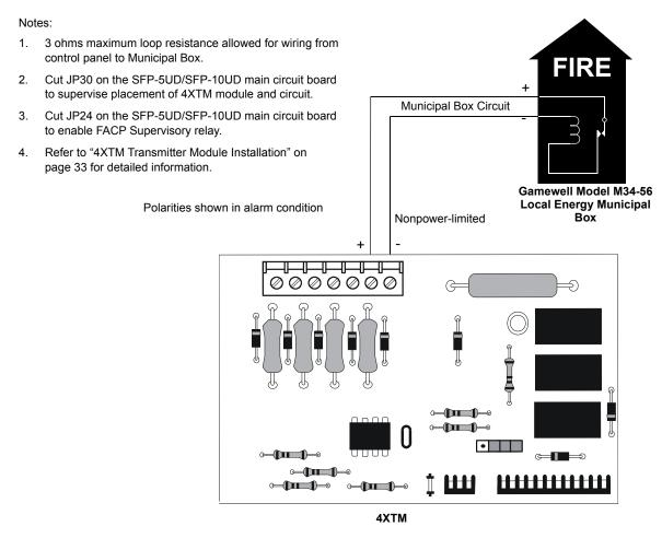
Figure B.2 Municipal Box Connected to 4XTM Transmitter Module
