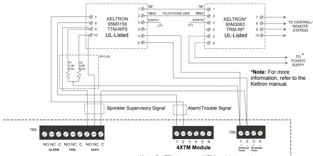
**Note:** Cut TBL jumper on 4XTM module to send alarm/trouble signal from the same pair or terminals.
