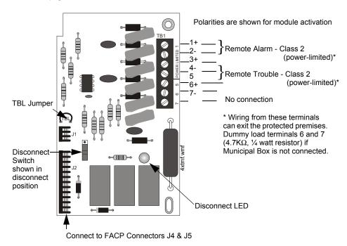
Figure 2.17 4XTM Transmitter Module
