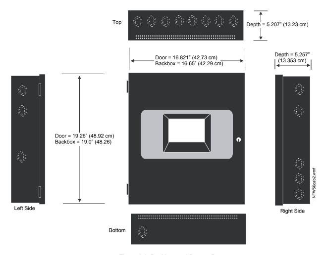
Figure 2.3 Backbox and Battery Box
