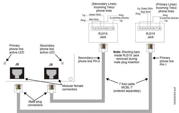
Figure 2.13 Wiring Phone Jacks
