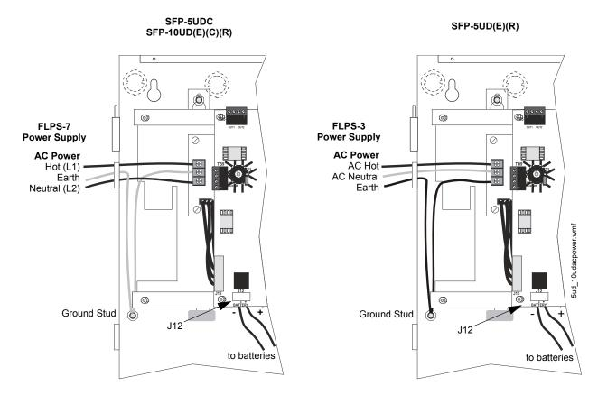
Figure 2.4 Operating Power Connections
