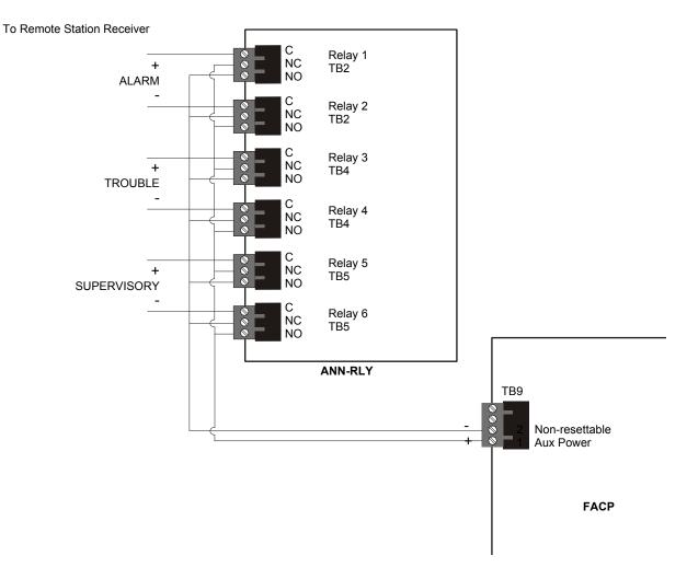
Figure F.2 Alternate Transmission for Alarm, Trouble, and Supervisory Signals
